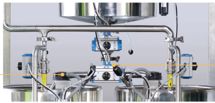
氣泡液位控制感知器 Bubble water level sensor
