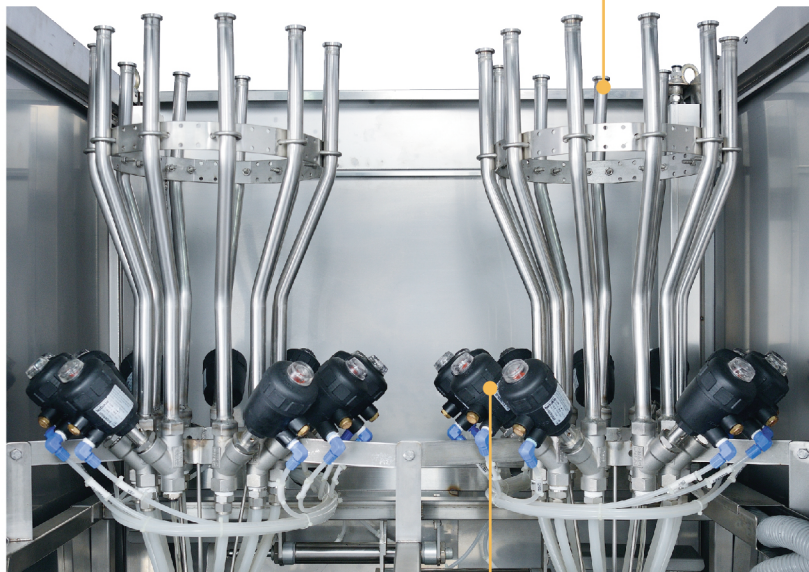
不銹鋼食品級管路助劑入口 Chemical inlet with stainless steel food grade tube
